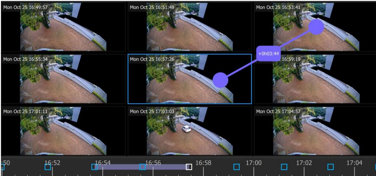
The search time frame selected by the mouse will reflect in the timeline at the bottom of the screen.
