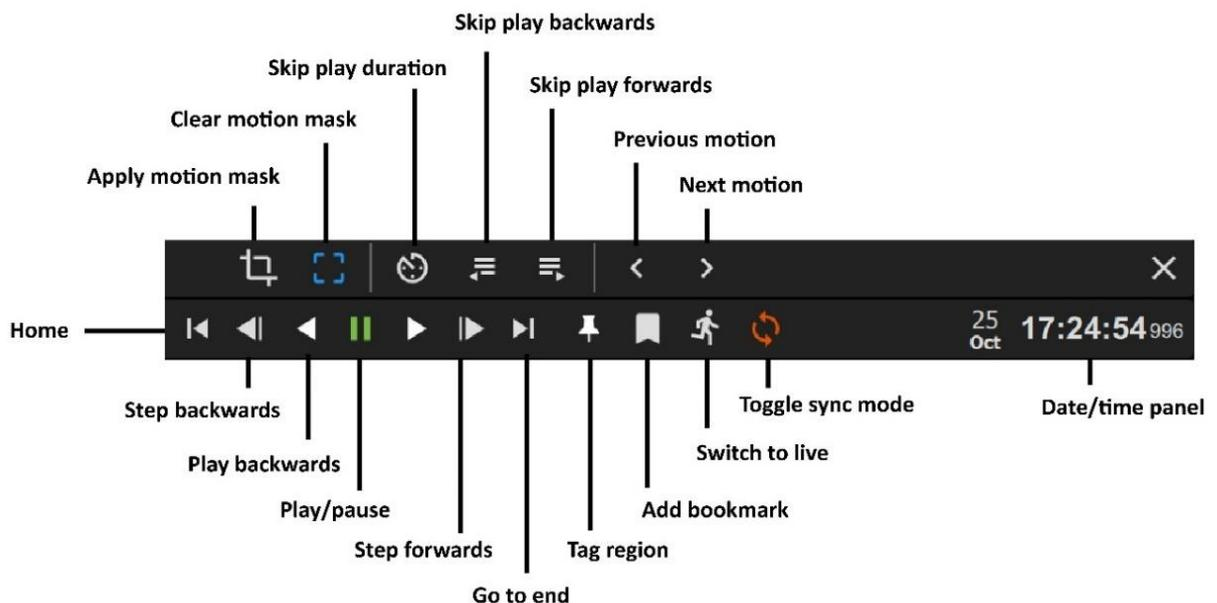
**Note:** Motion quick search is not available on all cameras. Although the *motion quick search controls* will open in the camera review panel for all cameras, when searching for next or previous motion, an error message will appear as shown below when this feature is not available.
