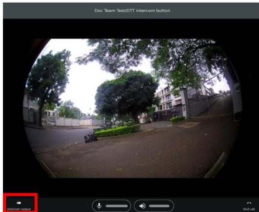
→ Click the intercom output button to toggle the relay output.
